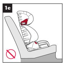
If one or both sections of the child seat are not in contact with both sections of the car's seat you MUST angle the car seat more upright (dia 1e).
